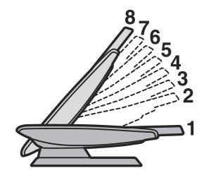
The angle of the operation board can be set to one of eight angles (level  $1 = 0^\circ$ , level  $8 = 45^\circ$ ).
