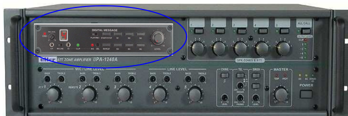
UDM-10 Installed in UPAS
